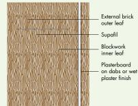
The systems shown do not require cavity barriers, and full-fill systems can be installed in all types of buildings across the built environment, as detailed in their British Board of Agrément (BBA) Certificates. With formal guarantees against liquid water penetration and a long history of use, they offer peace of mind for the specifier, builder and client alike.
