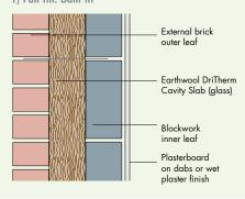
These systems not only provide the best U-value to wall width ratio but are also the lowest in cost. Even with dense concrete blocks it is possible to achieve very high thermal performance in a manageable wall width.
