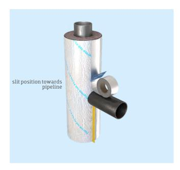
In order to connect the insulation segments tightly at the intersection, adjust the front surface of the pipe section to the outer radius of the already insulated pipe. In case of gaps use Thermo-teK Seal Cld and finish the installation with Therm-teK Tape Cld; use spatula.
