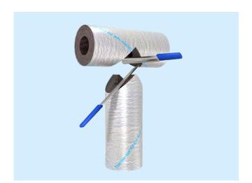
Place the pipe sections on the pipe line and close the longitudinal slits. Push both pre-cut pipe sections tightly together and seal the joint with the Thermo-teK Tape Cld. All tapes have to be smoothend and fastened with spatula, as described.
