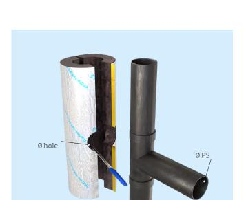
Use Thermo-teK Tape Cld to seal the intersection pipe in order to create a vapour barrier.
