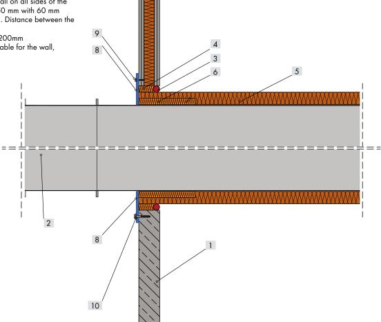
Application: Fire-teK® DuctProtect El 30 R **Fixation of the duct to the wall**one-sided fire classification requirements
