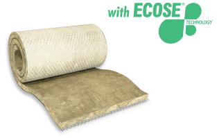
is supplied with a galvanised wire and galvanised mesh on one side, with white glass veil between mesh and mineral wool (GGV) for protection from dust/flocks, with max service temperature 640 or 660 °C, depending on density.
