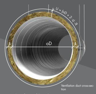
U = Circumference of the insulation in mm oD = External diameter of ventilation duct in mm s = Insulation thickness of wire mesh mat in mm
