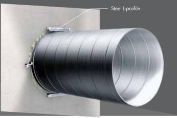
The gap between the ventilation duct and fire wall/ceiling must be filled with mineral wool (density:  $\geq 80 \, \text{kg/m}^3$ ). Finally, cover the gap on both sides with a fire safety sealing compound, layer thickness approx. 5 mm.
