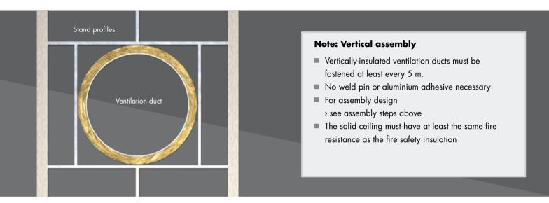
In a drywall, the under-construction is adjusted in the intersection area as shown in the illustration. The drywall must have at least the same fire resistance as the fire safety insulation.
