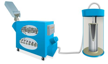
In the **blowing machine**, flocks are fed to the hopper. The feeder transfers flocks to the shredder, while the stream generated by the blower conveys the insulation to the outlet at high speed (air flow and insulation flow can be
