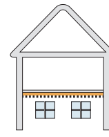
Basement rooms with lined floor joist
