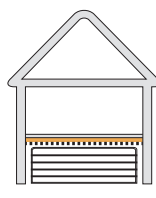
Garage with lined floor joist
