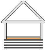
Sub-floor with timber battens
