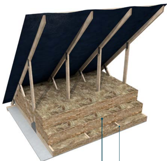
Ceiling Roll — between and above ceiling joists
