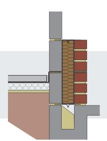
DriTherm® Cavity Slabs can be used in situations where they bridge the DPC in walls. Tests by the British Board of Agrément confirm that DriTherm® Cavity Slabs will not transmit water to the inner leaf, nor will they transmit moisture by capillary action across the cavity or from below damp proof course level provided they are installed correctly.
