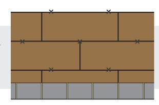
Where cavity insulation batts or slabs start below DPC level, the vertical and horizontal spacing of wall ties should be compatible with the spacing to be used above DPC level.
