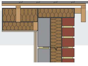
Cavity trays should remain clear of droppings and debris.
