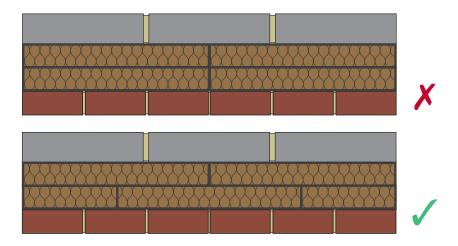
It is recommended that mineral wool batts with a thickness of 75mm or less are bent around corners to ensure that no gaps are left between batts, into which mortar could fall. Otherwise ensure joints are closely butted.
