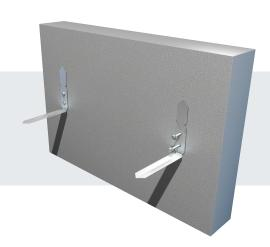
Brackets should be positioned at maximum 500mm centres, approximately 150mm in from each end. Cut areas of slab should use two brackets if larger than 200mm long, and one bracket located centrally if less than 200mm long. Do not but multiple short pieces together.
