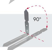
Once bent, the bracket can be fixed back to the inner leaf, using at least two bolts to provide a secure fixing. Ensure noncombustible fixings suitable for the substrate are used.
