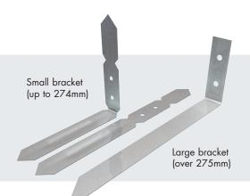
If using the small bracket, bend the bracket so that either the large or small pointed section is at 90 degrees depending on the depth of the barrier. Use the small leg if the barrier is up to 90mm and the large leg if the barrier is 91-274mm.
