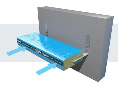
At the end of a run of barriers, or at corners, the barrier should butt up to the outer leaf.
