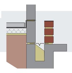
Position the Rocksilk® RainScreen Slab against the inner leaf. The slabs should be cut to size if necessary and should be taken below the floor insulation to reduce thermal bridging, with no risk of capillary action. Rocksilk® RainScreen Slab does not wick moisture and is suitable for use below DPC. Always ensure that Rocksilk® RainScreen Slab is course with wall ties.
