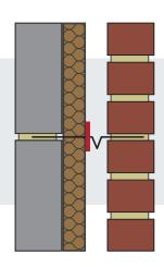
Rocksilk® RainScreen Slab is supplied for use in partially filled masonry cavities in 1200 x 455mm slabs for use between wall ties at 450mm vertical centres.
