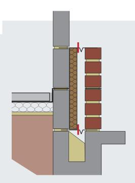
Wall ties should be built into joints, not pushed and positioned, so that the drip faces downwards and the ties are level or slope slightly towards the outer leaf.
