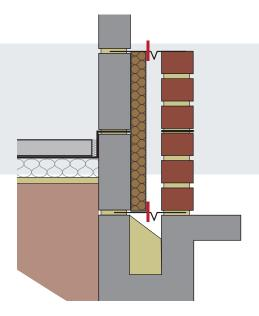
Proceed similarly with successive stages of the wall. As with normal masonry cavity wall constructions, no mortar should remain in the cavity, particular care should be taken to keep slab joints closely butted and free from mortar. To facilitate keeping the top edges of slabs clean it is recommended that cavity boards be used.
