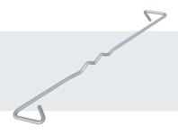
Generally, rows of wall ties should be at 450mm vertical spacing and at horizontal spacings of no more than 900mm or as otherwise required by the structure. Where whole rows of ties are at different vertical spacings Rocksilk® RainScreen Slab should be cut to course, allowing an extra 5mm for compression to form close butt joints.
