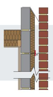
Cavity trays should remain clear of droppings and debris. Rocksilk® RainScreen Slab can be easily cut to a chamfer to suit the profile of the cavity tray and ensure no voids are present in the cavity. Slabs can be easily cut with a sharp knife or saw to suit.
