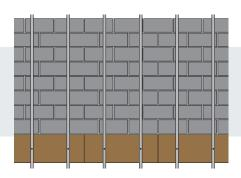
From above, slide the next row of Rocksilk® RainScreen Slab into place behind the brick tie channel. The slabs will be retained in position by the channel and supported by the row of slabs below.
