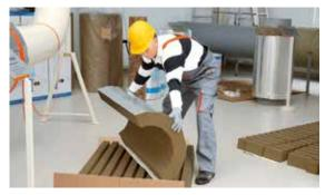
Delivered flat on pallets the material is easy to store and handle — even if space on site is limited. A half shell can be immediately built when the trapezoid-belt is taken from the package.
