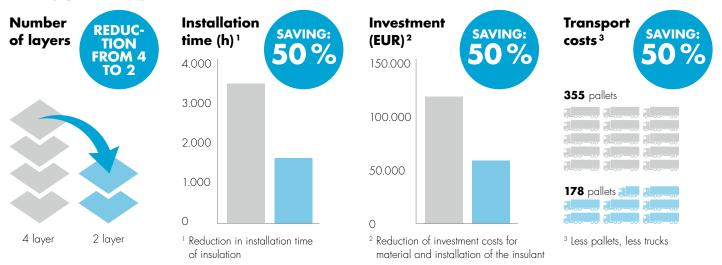
4 layer Mineral Wool boards 35 kg/m³ 2 layer Power-tek RL 220
